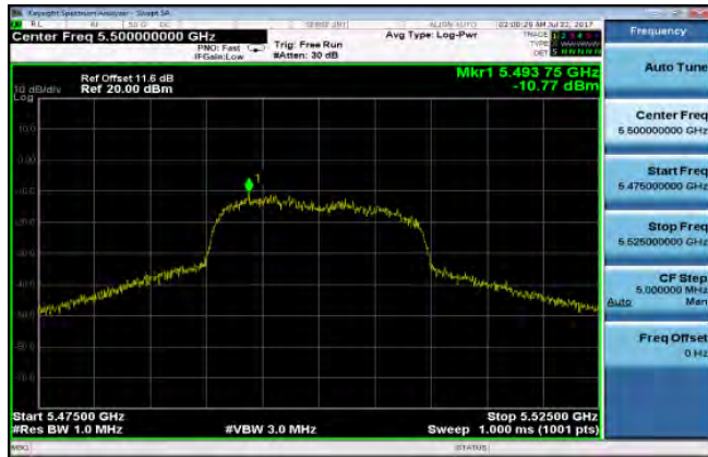
Peak Power Spectral Density Data Plot (CH Mid 5580MHz)
