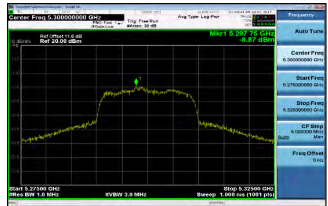
Peak Power Spectral Density Data Plot (CH High 5320 MHz)
