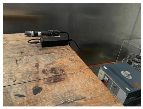
Test setup photo for radiated emission test (30MHz-1GHz)
