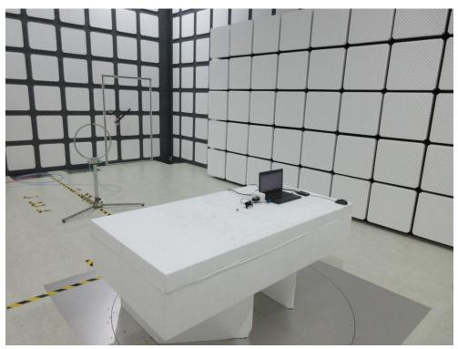
Test Mode: Mode 1 Description: Radiated Emission Test Setup for below 1GHz
