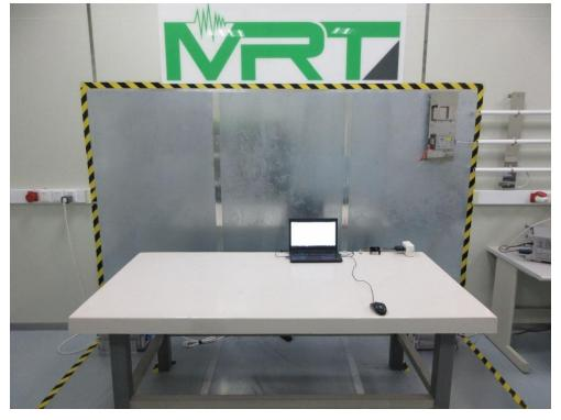
Test Mode 2 Description: Back View of Conducted Emission Test Setup
