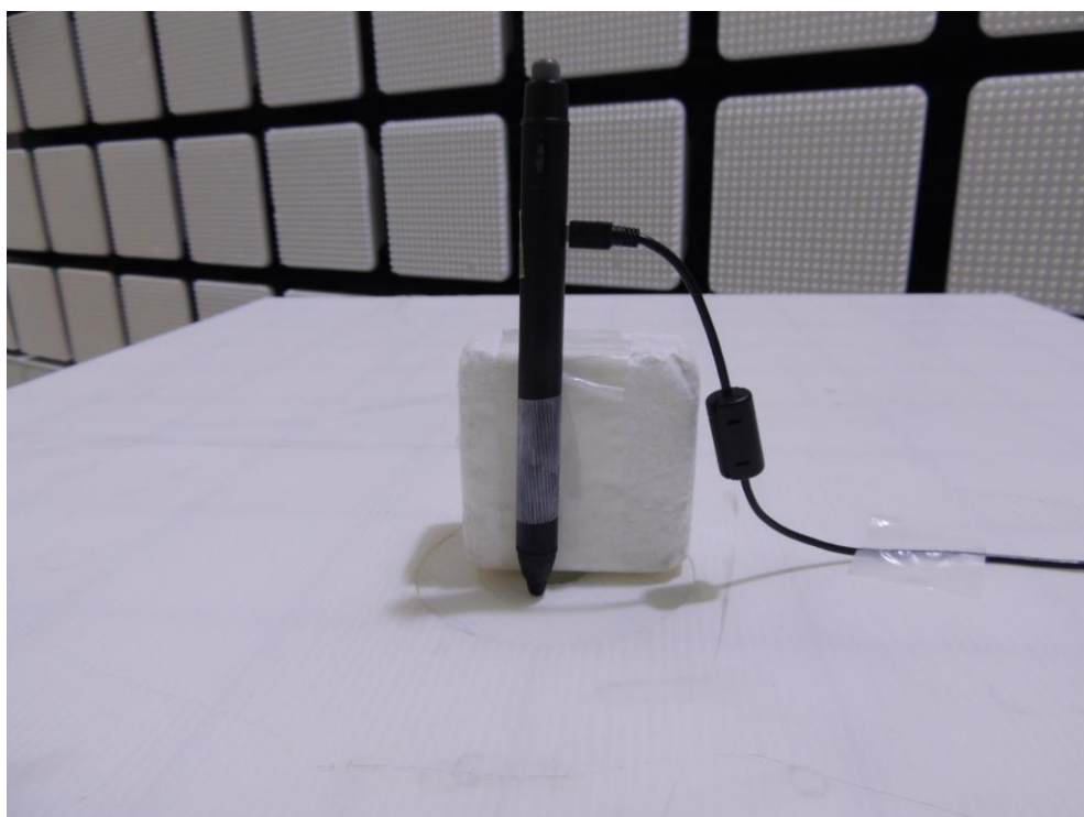
Photograph 6: Set-up for Radiated Emission, EUT Configuration Z-Axis
