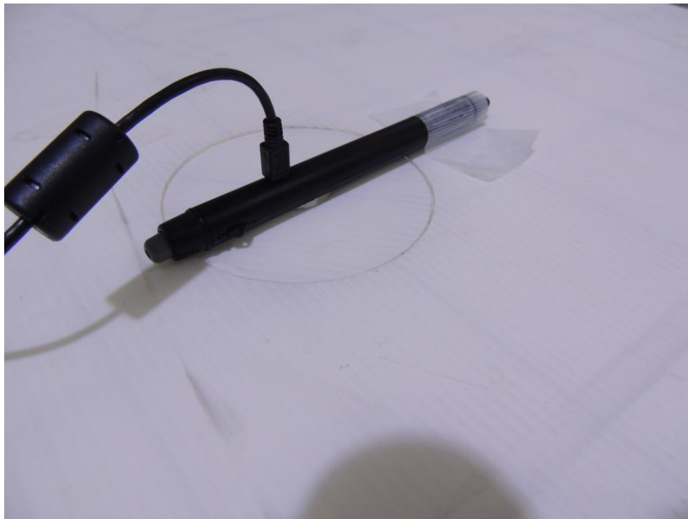
Photograph 5: Set-up for Radiated Emission, EUT Configuration Y-Axis
