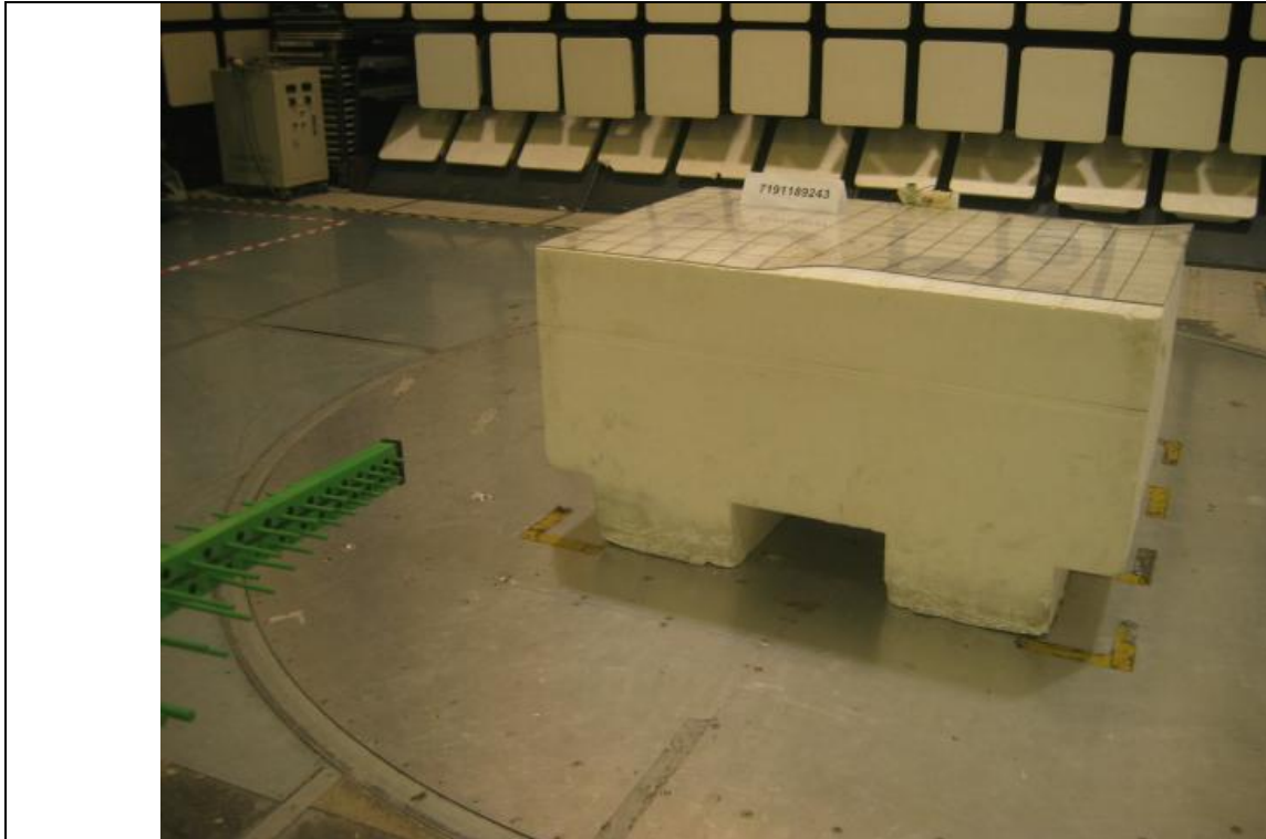
Radiated Emissions (Spurious Emissions Inclusive Restricted Bands Requirement) Test Setup (Front View)
