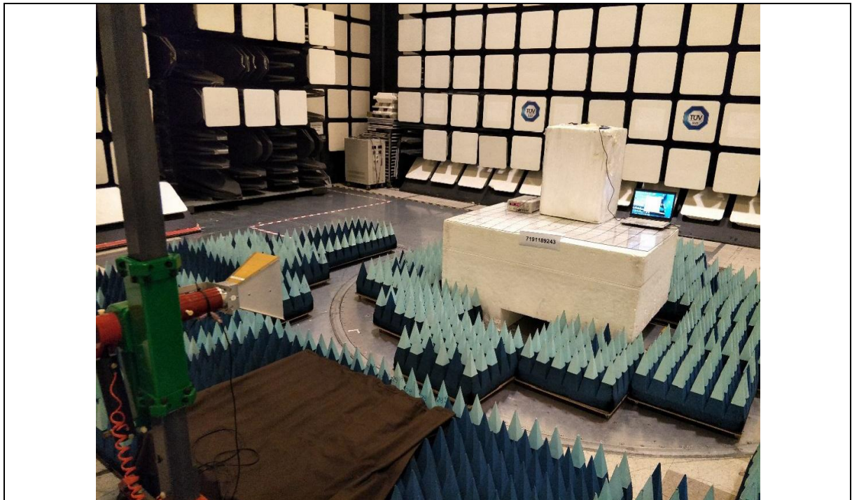
Radiated Emissions (Spurious Emissions Inclusive Restricted Bands Requirement) Test Setup (Front View)
