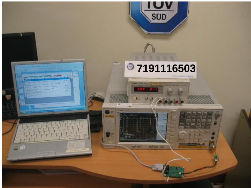
Number of Hopping Frequencies Test Setup
