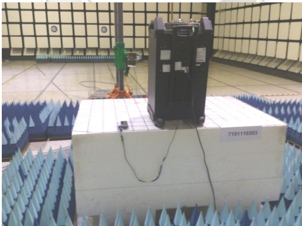
Band Edge Compliance (Radiated) Test Setup
