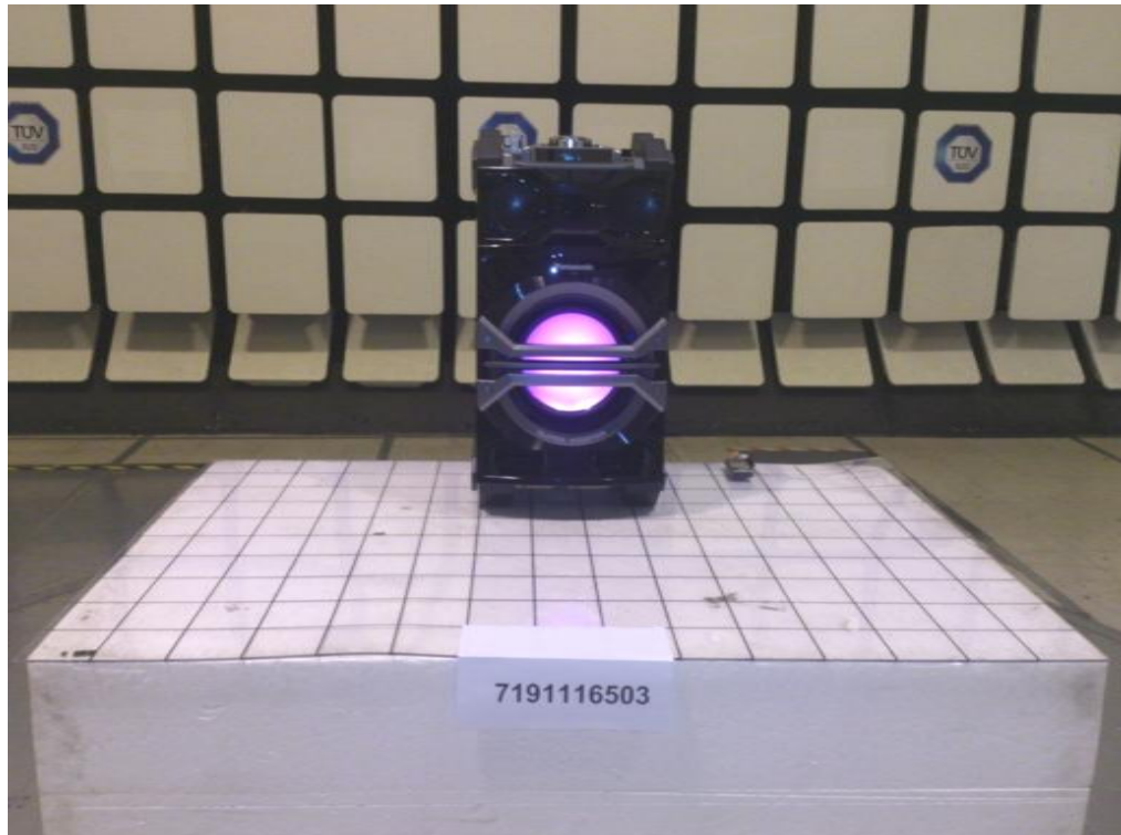
Radiated Emissions Test Setup (Front View)
