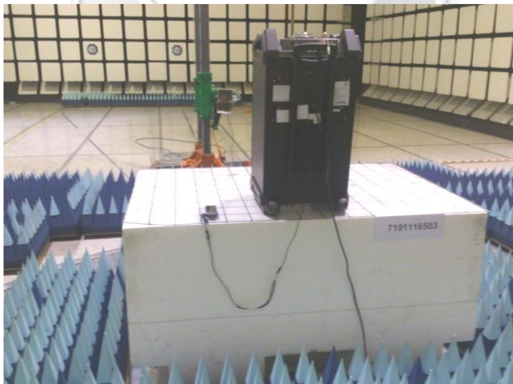
Radiated Emissions Test Setup (Rear View)
