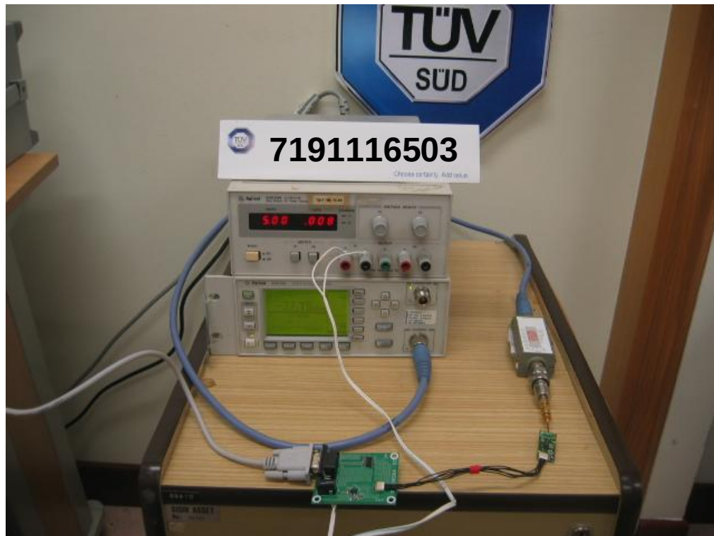
Maximum Peak Power Test Setup
