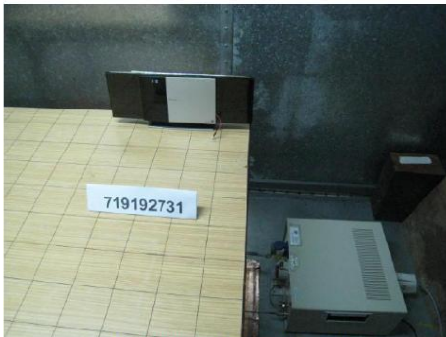
Conducted Emissions Test Setup (Front View)
