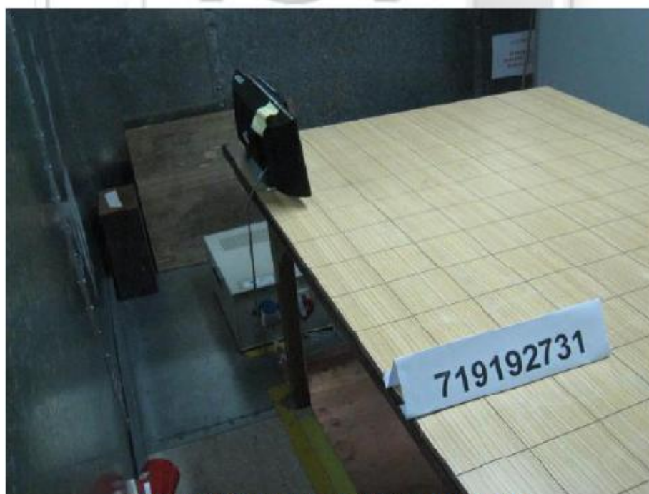
Conducted Emissions Test Setup (Rear View)
