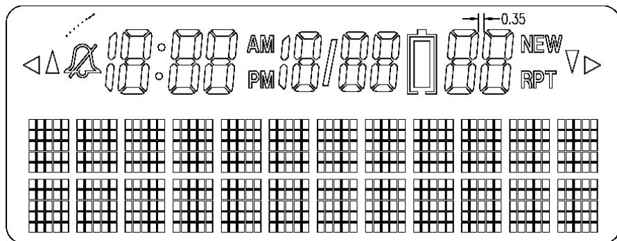
The display is controlled by pins 13 – 70 of MCU.
