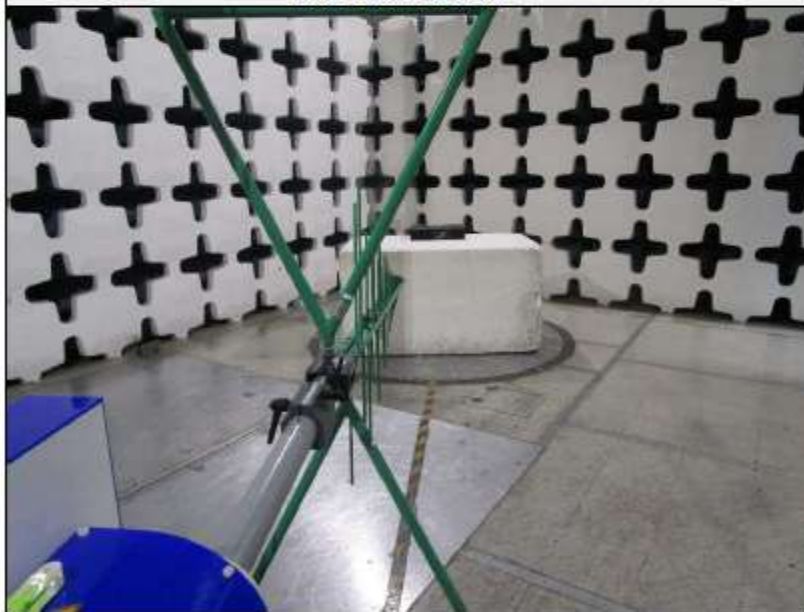
Test Setup for Spurious Radiated Emissions, 30MHz – 1GHz – Antenna Polarization Vertical
