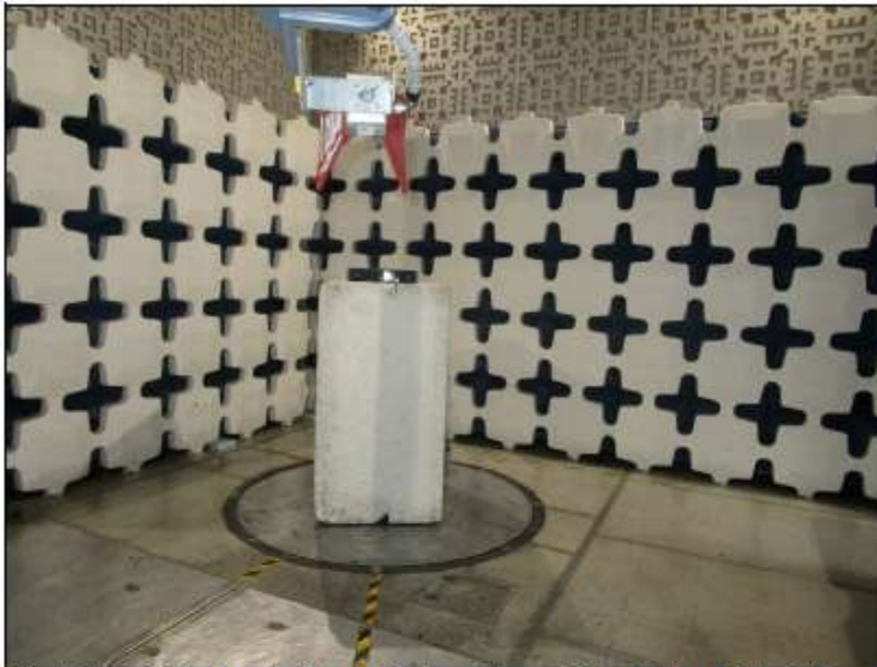
Test Setup for Spurious Radiated Emissions, Above 1GHz – Antenna Polarization Horizontal
