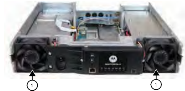
Figure 4: Front view (without top and bottom covers) of the SLR 8000 Base Station/Repeater
