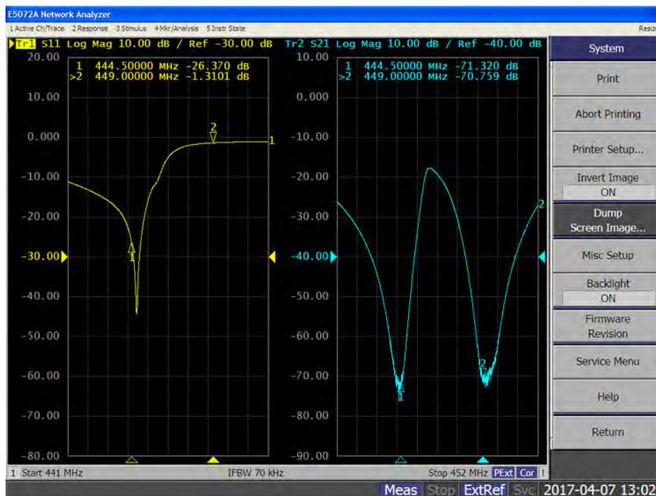
Figure 27: Rejection of Each Port for UHF Duplexer
