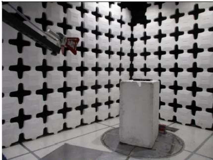
Test Setup for Spurious Radiated Emissions, Above 1GHz – Antenna Polarization Horizontal
