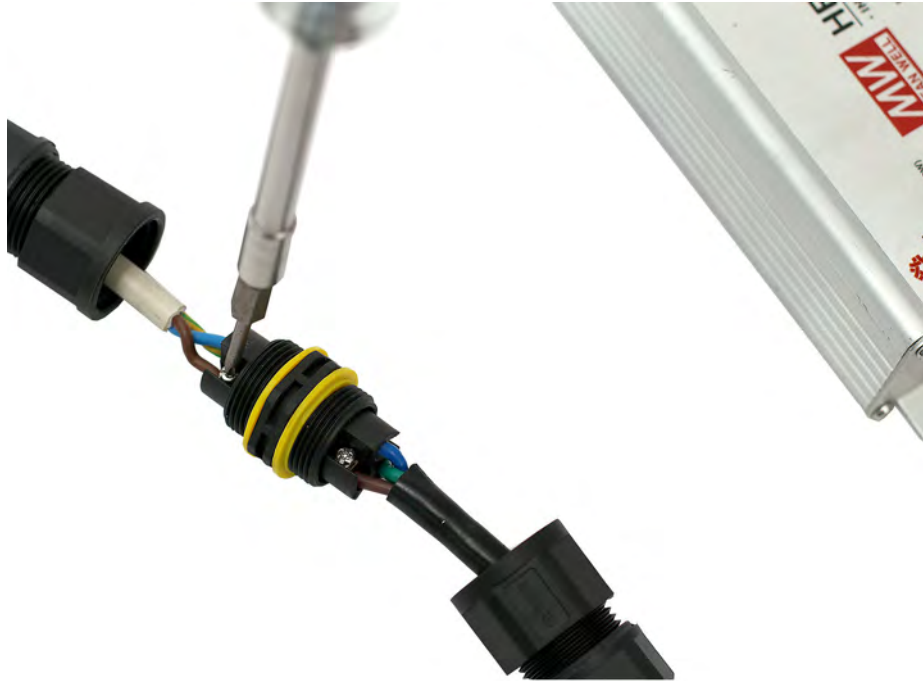
Figure 42: Attach AC Wires to Joiner A
