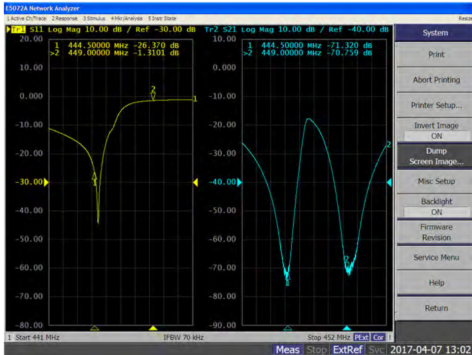
Figure 27: Rejection of Each Port for UHF Duplexer
