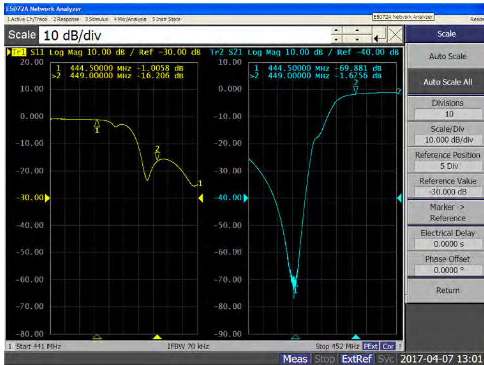
Figure 25: Example for HIGH Port Tuning of the UHF Duplexer
