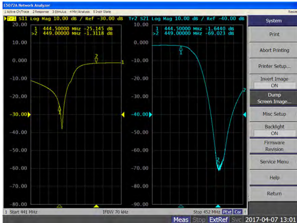
Figure 26: Example for LOW Port Tuning of the UHF Duplexer
