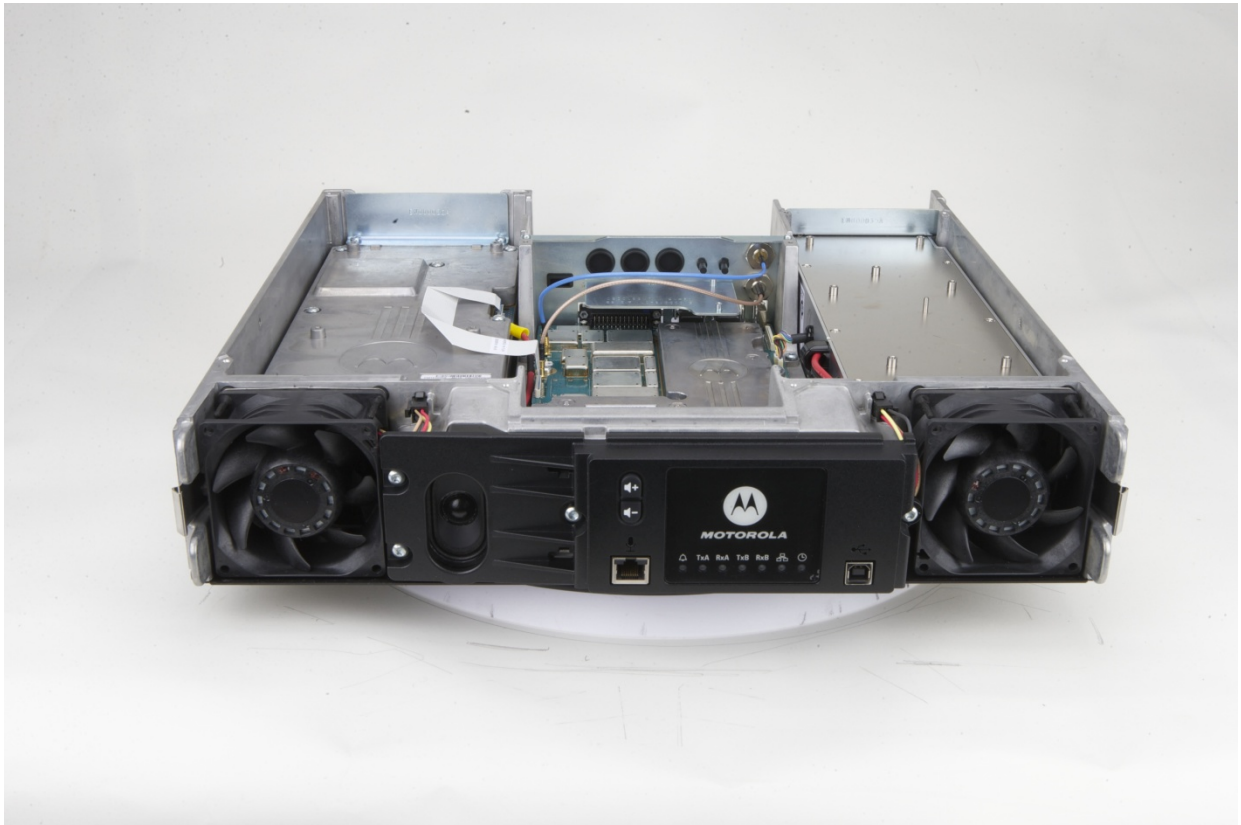
External Front View of Base Radio, Top Cover and Front Panel Removed
