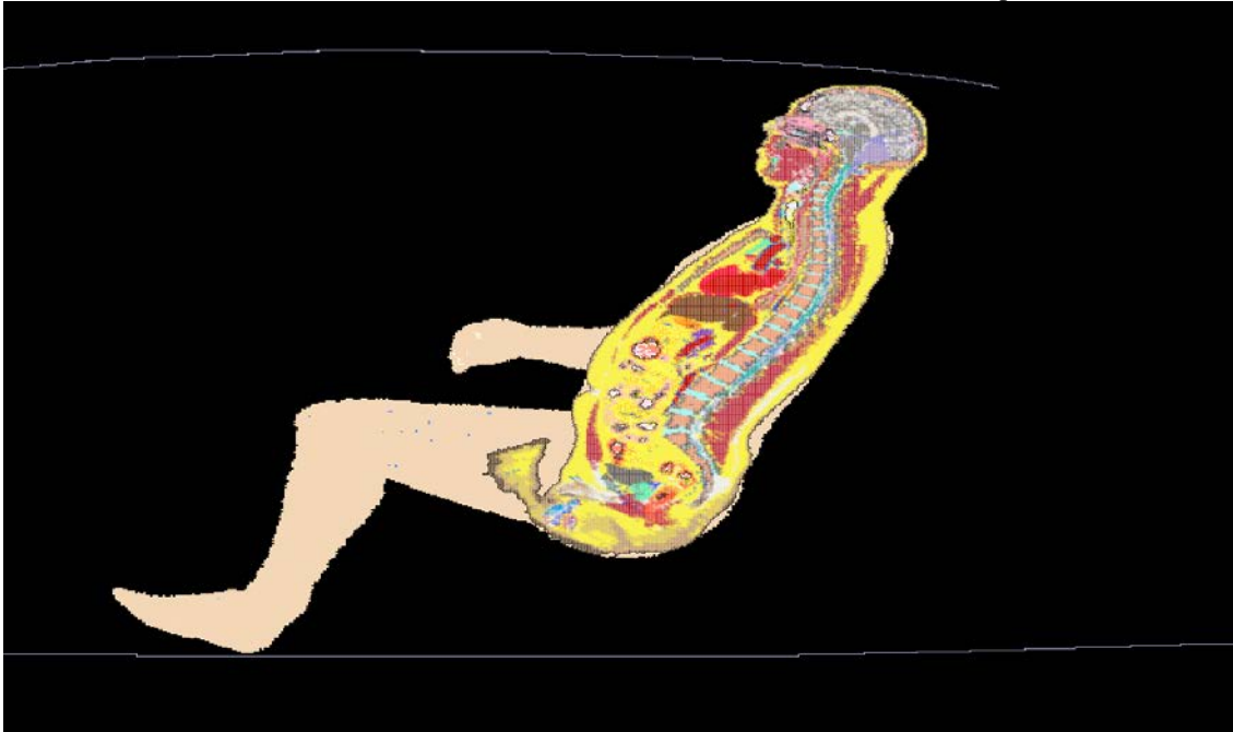
Figure 2: Passenger model exposed to a trunk-mount antenna: XFDTD geometry. The antenna is mounted at 85 cm from the passenger located in the center of the back seat.
