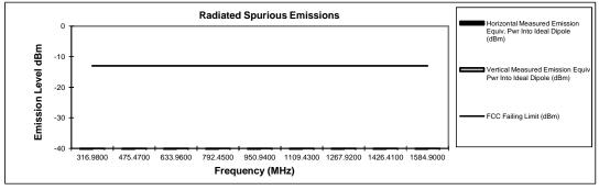
Transmit Radiated Spurious Emissions: PMUD3240AABNAA Tx Power: 54 Watts
