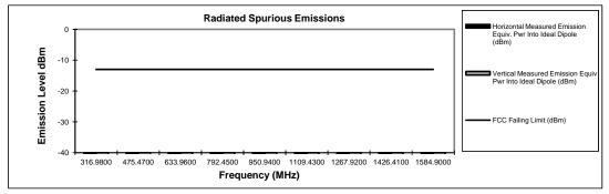
Transmit Radiated Spurious Emissions: PMUD3240AABNAA Tx Power: 25 Watts
