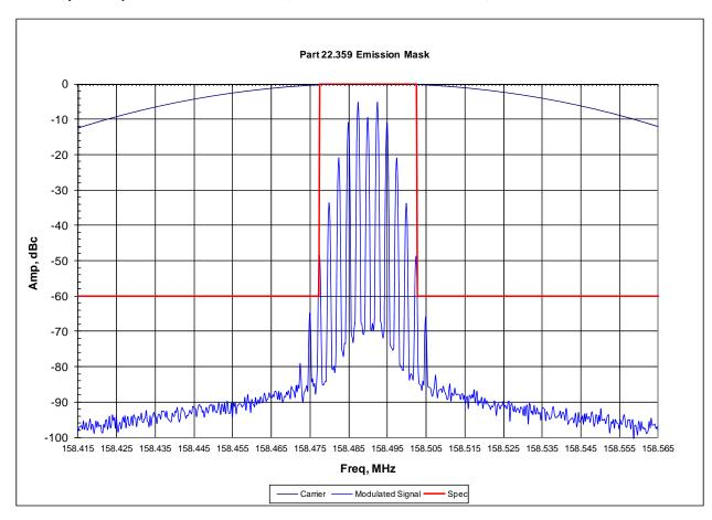
158.490 MHz CENTER FREQUENCY: 300 Hz RESOLUTION BANDWIDTH: VIDEO BANDWIDTH: 1 kHz SPAN: 150 kHz DETECTOR MODE: **AVG** HORIZONTAL SCALE: 10 kHz/div SWEEP TIME: 50 Sec. VERTICAL SCALE: 10 dB/div
