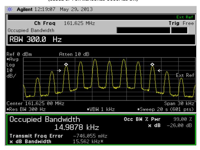
CENTER FREQUENCY: 161.625 MHz RESOLUTION BANDWIDTH: 300 Hz VIDEO BANDWIDTH: 1 kHz SPAN: 30 kHz DETECTOR MODE: AVG HORIZONTAL SCALE: 3 kHz/div SWEEP TIME: 20 Sec. VERTICAL SCALE: 10 dB/div
