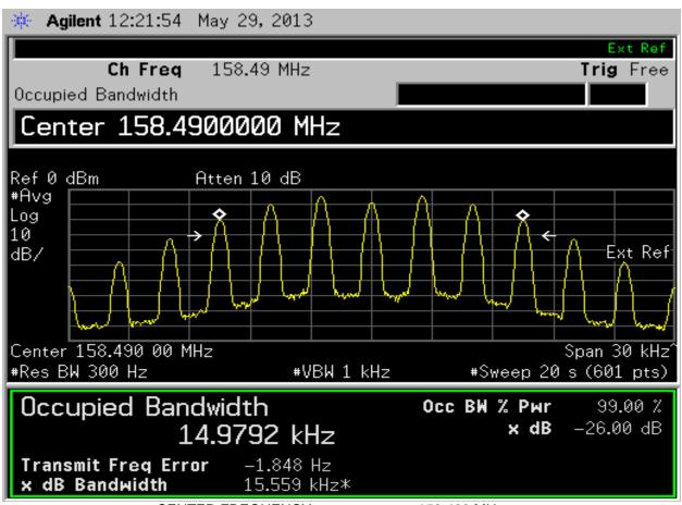
CENTER FREQUENCY: 158.490 MHz RESOLUTION BANDWIDTH: 300 Hz VIDEO BANDWIDTH: 1 kHz SPAN: 30 kHz DETECTOR MODE: AVG HORIZONTAL SCALE: 3 kHz/div SWEEP TIME: 20 Sec. **VERTICAL SCALE:** 10 dB/div
