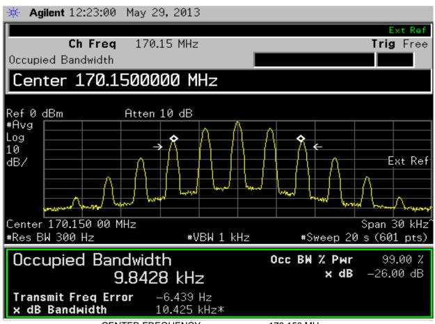
170.150 MHz CENTER FREQUENCY: RESOLUTION BANDWIDTH: 300 Hz VIDEO BANDWIDTH: 1 kHz SPAN: 30 kHz DETECTOR MODE: **AVG** HORIZONTAL SCALE: 10 kHz/div SWEEP TIME: 20 Sec. VERTICAL SCALE: 10 dB/div
