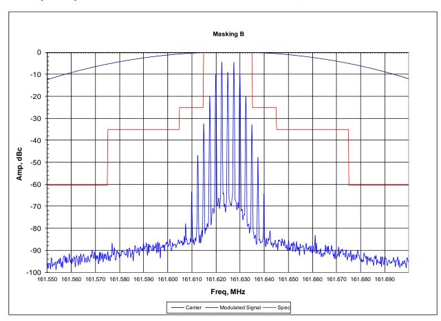
161.625 MHz CENTER FREQUENCY: **RESOLUTION BANDWIDTH:** 300 Hz VIDEO BANDWIDTH: 1 kHz SPAN: 150 kHz **DETECTOR MODE: PEAK** HORIZONTAL SCALE: 10 kHz/div SWEEP TIME: 50 Sec. VERTICAL SCALE: 10 dB/div
