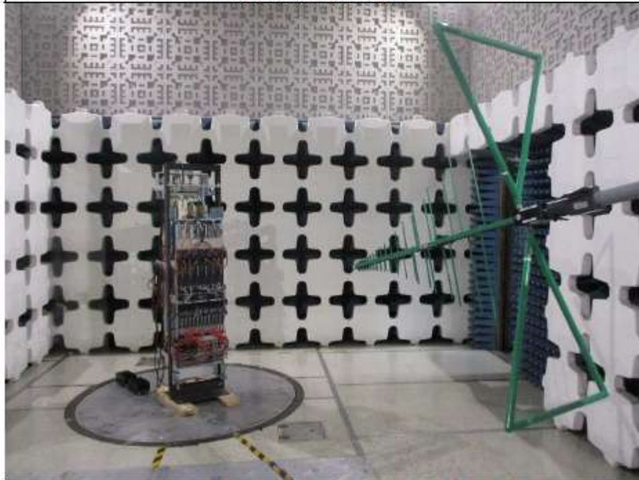
Test Setup for Case Spurious Radiated Emissions, 30MHz – 1GHz – Antenna Polarization Vertical
