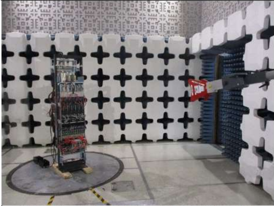
Test Setup for Case Spurious Radiated Emissions, Above 1GHz – Antenna Polarization Horizontal
