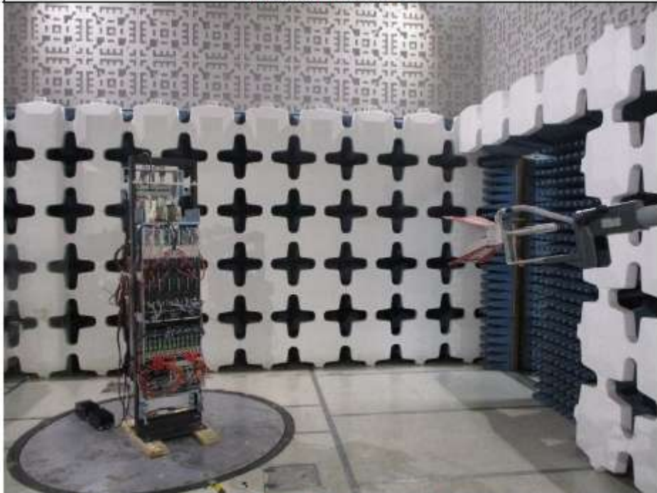
Test Setup for Case Spurious Radiated Emissions, Above 1GHz – Antenna Polarization Vertical
