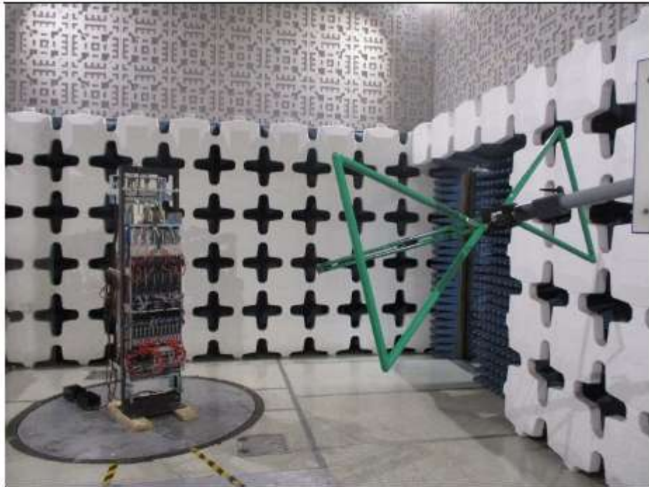
Test Setup for Case Spurious Radiated Emissions, 30MHz – 1GHz – Antenna Polarization Horizontal
