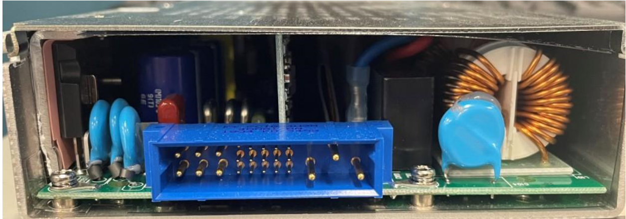
D3-3 Internal Back View – Transceiver Power Supply Module
