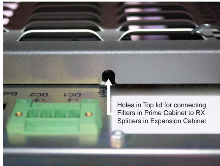
Figure 65: Holes in Top Lid for Rx Cables
