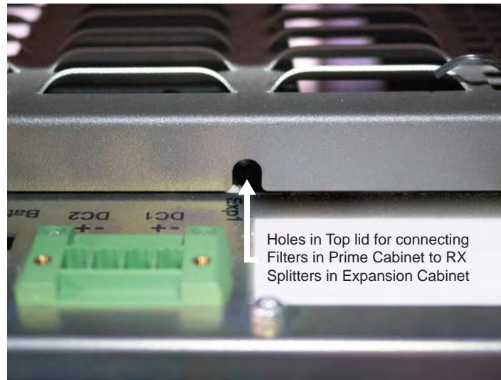
Figure 118: Holes in Top Lid for Rx Cables
