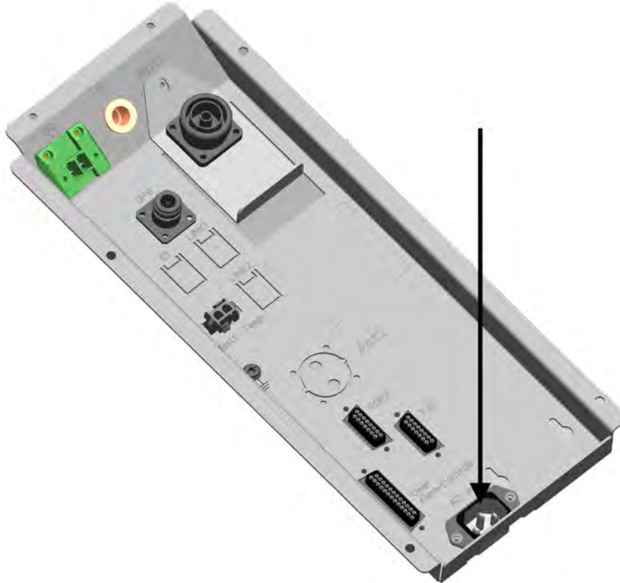
Figure 39: 100–240 VAC Connection on the MTS LiTE Junction Panel
