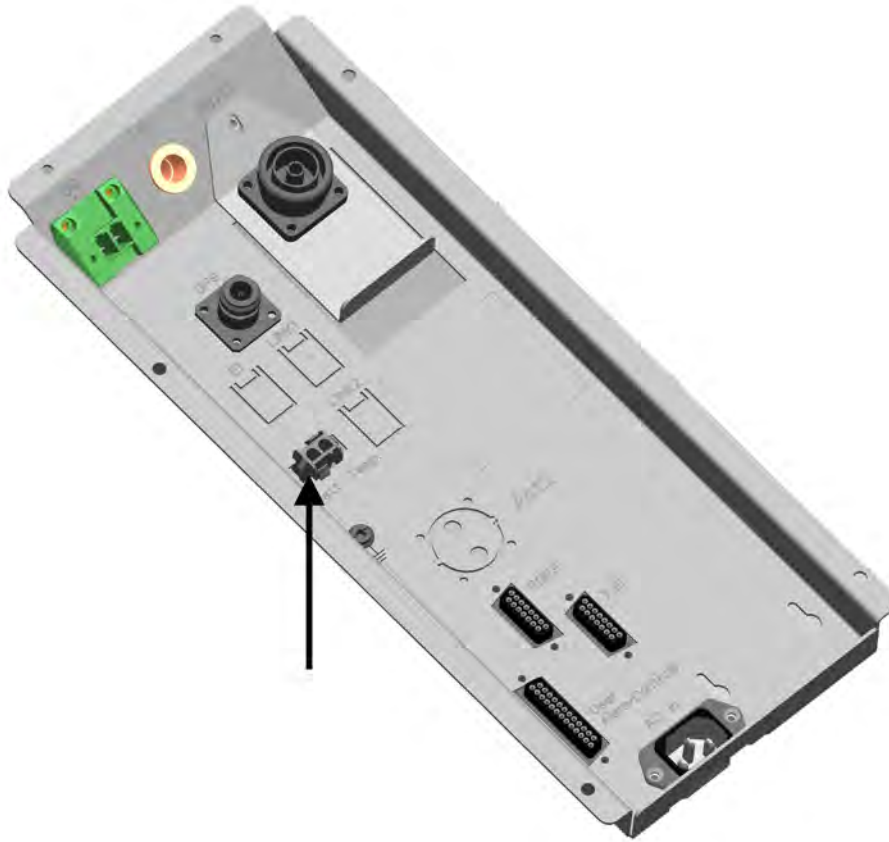
Figure 44: Backup Battery Sensor Connection on MTS LiTE Junction Panel
