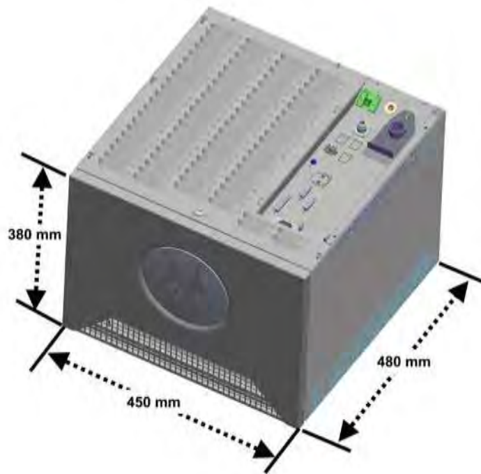
Figure 5: MTS LiTE Cabinet Dimensions
