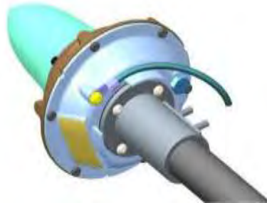
Figure 218: GNSS Antenna Assembly – Grounding Cable
