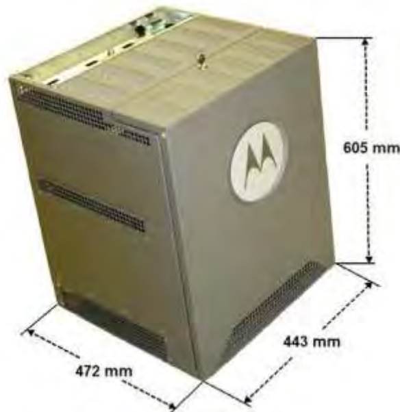
Figure 7: MTS 2 Cabinet Dimensions
