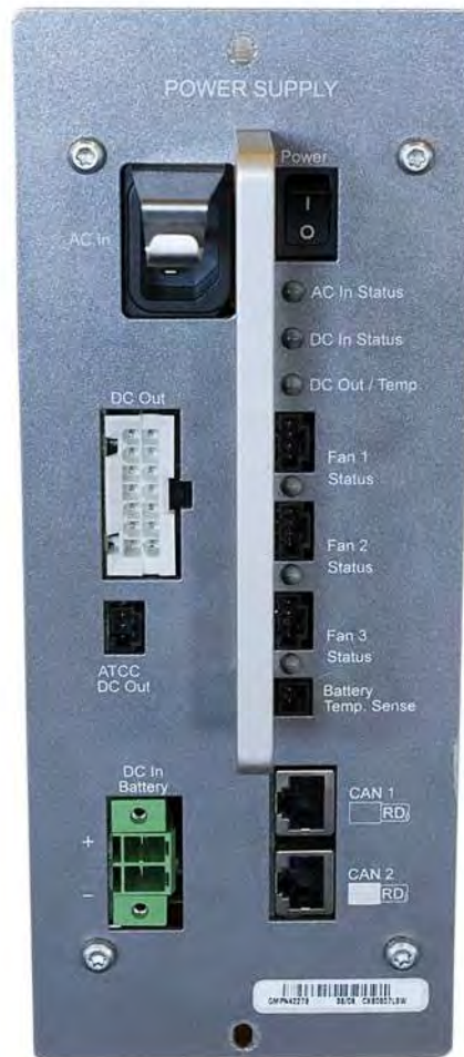
Figure 183: Power Supply Unit Front Panel
