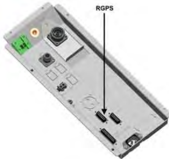
Figure 66: Remote GPS Receiver Connection on MTS 2 Junction Panel
