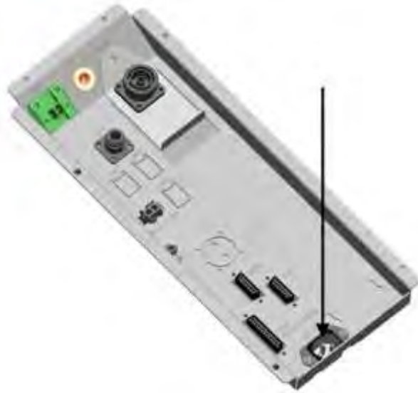
Figure 39: 100–240 VAC Connection on the MTS 2 Junction Panel
