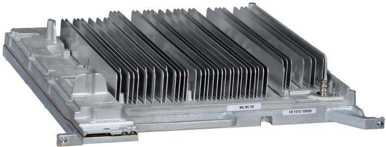
Internal Back View – Power Amplifier Module
