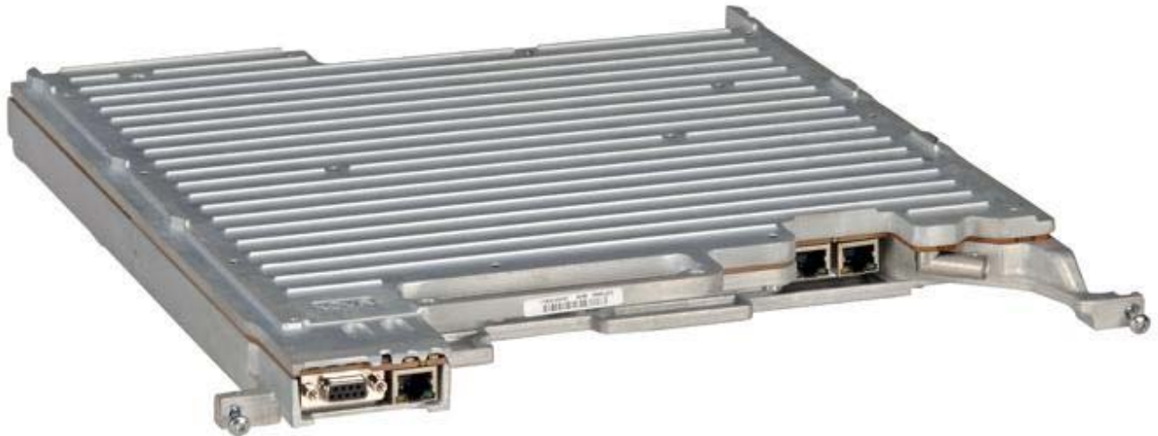
Transceiver Module without the Transceiver Option Card (TOC)
