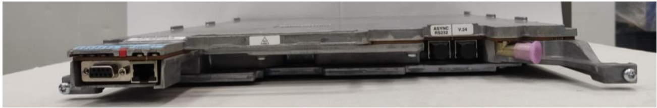
Transceiver Module without the Transceiver Option Card (TOC)
