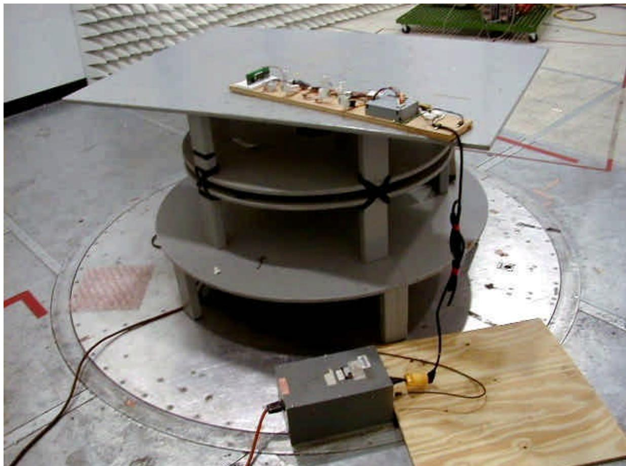
**Line Conducted Emissions Test Configuration**
