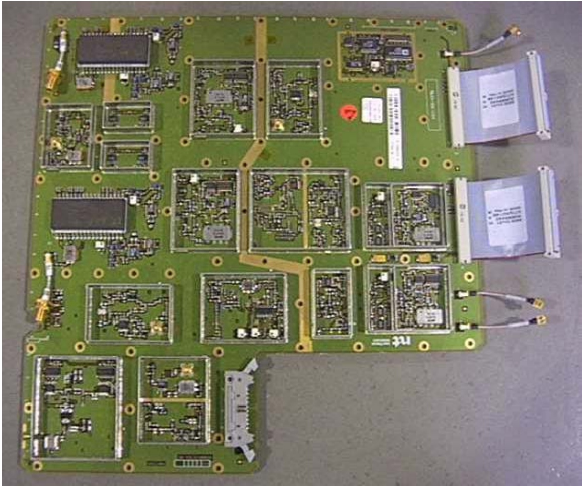
Figure 11 – RDRX 1900 MHz (Radio Board) Top View
