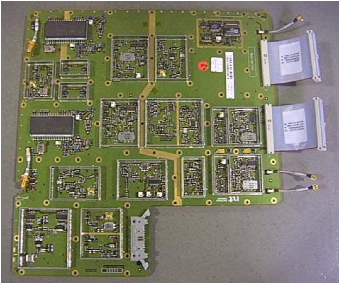
Figure 11 – RDRX 1900 MHz (Radio Board) Top View
