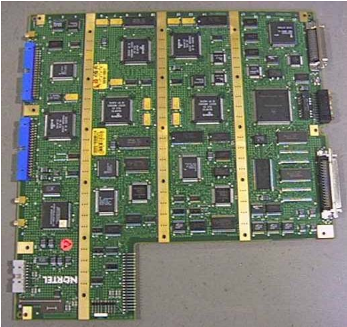
Figure 9 – LDRX 1900 MHz (Logic Board) Top View
