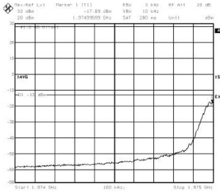
Figure 5 : -1 MHz adjacent band (Channel 737, Pmax - 4 dB) Diplexer only, GMSK modulation
