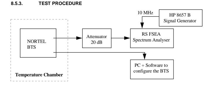
The BTS was configured to transmit at maximum power (static level 0). At each temperature, measurements were made with the primary supply voltage of the nominal value. At each of the above specified conditions, the maximum carrier frequency deviation was recorded from the time the transmitter was keyed-on for a period of ten minutes using a R&S FSEA spectrum analyzer.
