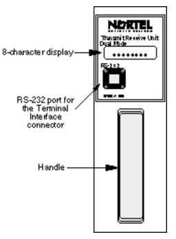
Figure 11-2 Front panel layout of the TRU3 (NTAW99AA)
