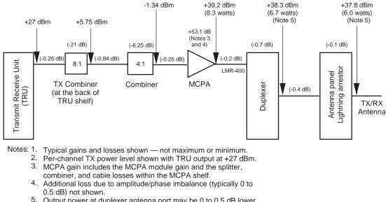
Output power at duplexer antenna port may be 0 to 0.5 dB lower due to amplidtue/phase imbalance.
