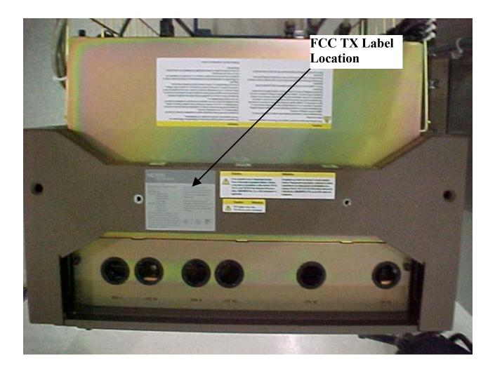
Nortel Networks Indoor Dual Mode Urban AB6NTL100AA FCC TX ID Label Location (Top View)
