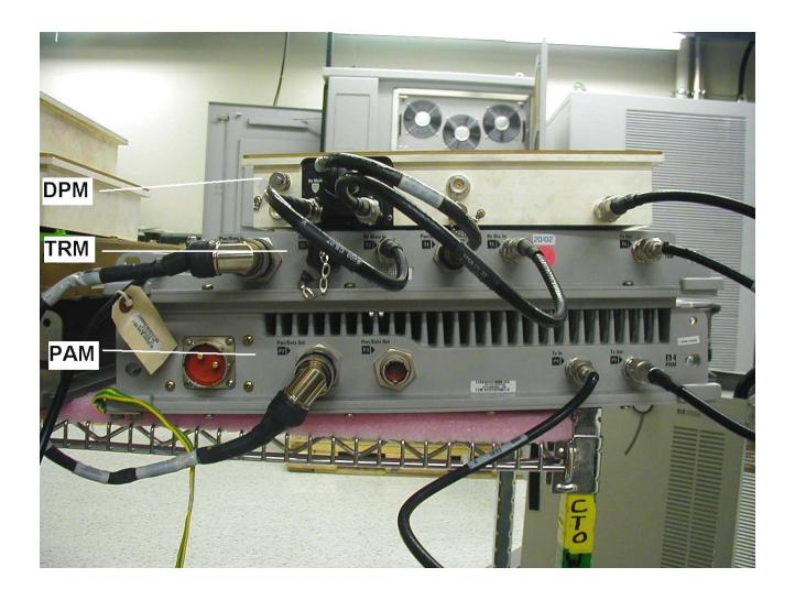
Nortel Networks SFRM Assembly Front View Fan Assembly Removed
