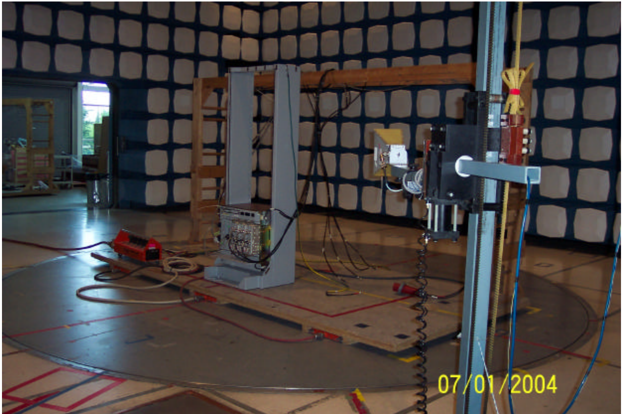
Figure 2 RE 1 GHz – 18 GHz EUT Configuration
