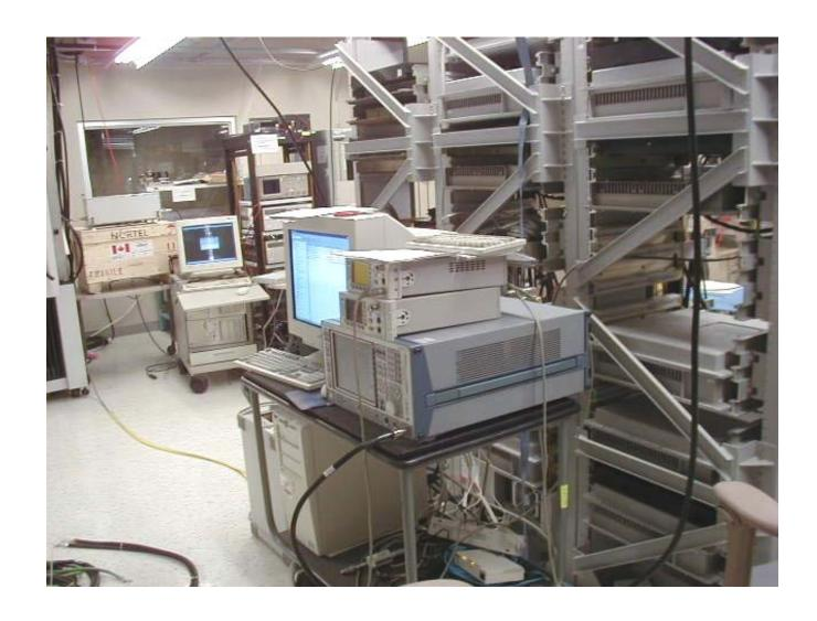
Test setup for the Spurious Emission at Antenna Terminals
