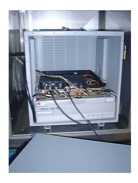
Test setup for the Spurious Emission at Antenna Terminals
