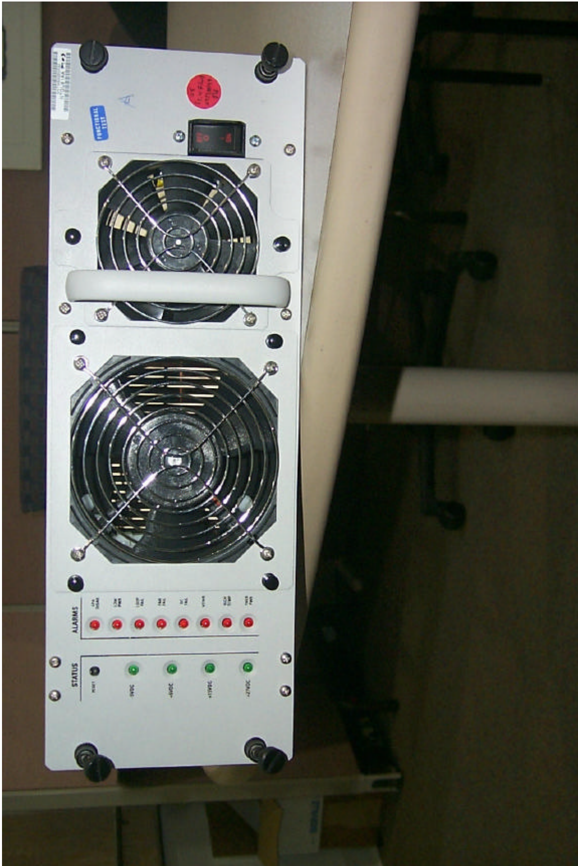
Nortel 800 MHz Flexible Radio Module AB6NT800EFRM Powerwave amplifier (FCC ID# E675JS0035) Front view
