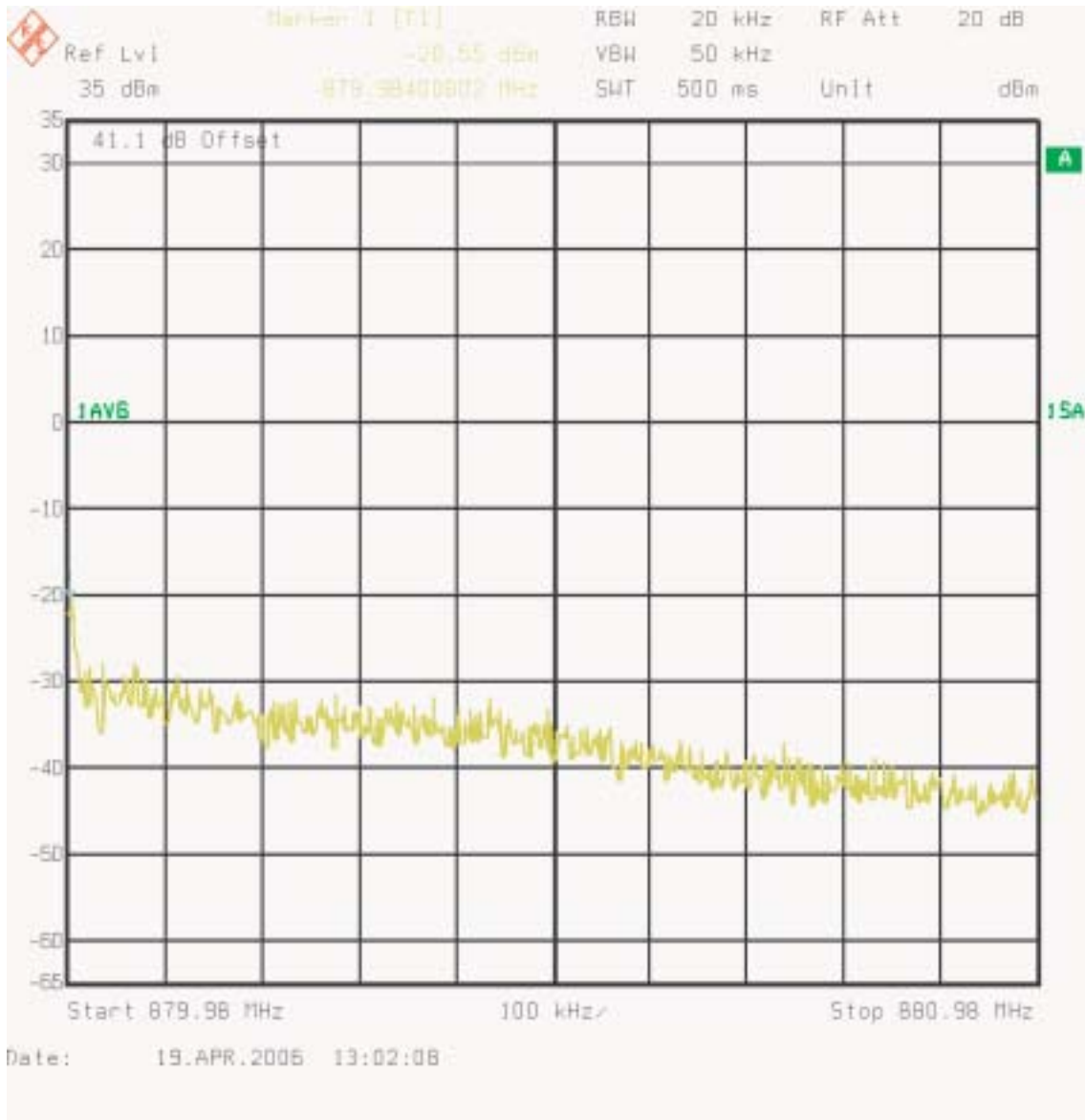
Figure 10 : 1 Carrier - Upper Adjacent Channel 1MHz Channel 308
