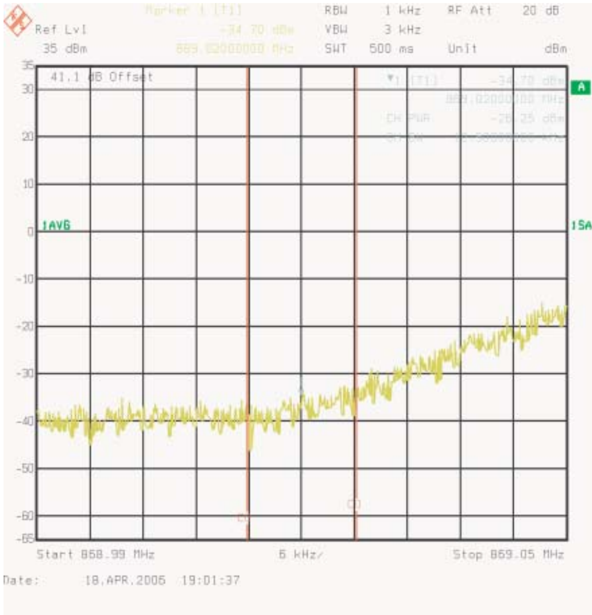
Figure 9 : One Carrier - Ch1015 IS95 Lower A" Band Adjacent to outside edge 12.5kHz band Channel Power
