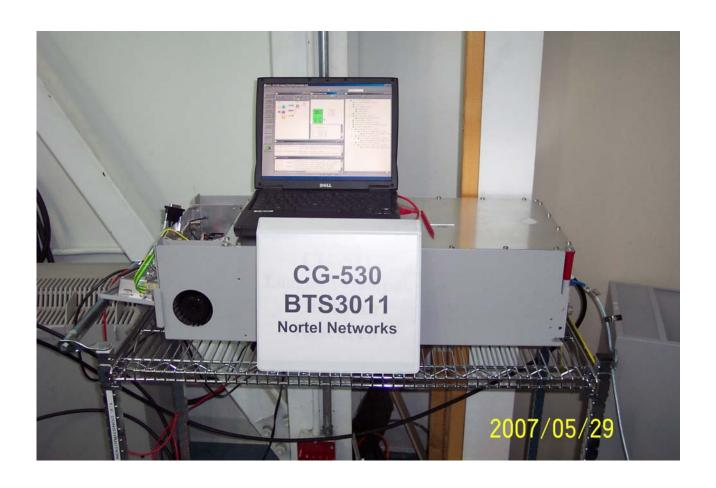
Test setup for the Spurious Emission at Antenna Terminals
