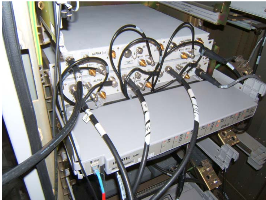
Figure 2. LTE MFRM3 1.7/2.1GHz. Conducted Spurious Emissions Antenna Port. EUT Setup
