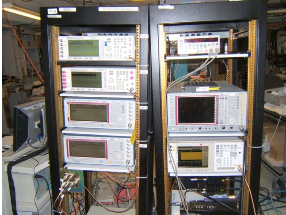
Figure 1. LTE MFRM3 1.7/2.1GHz. Conducted Spurious Emissions Antenna Port. Test Setup
