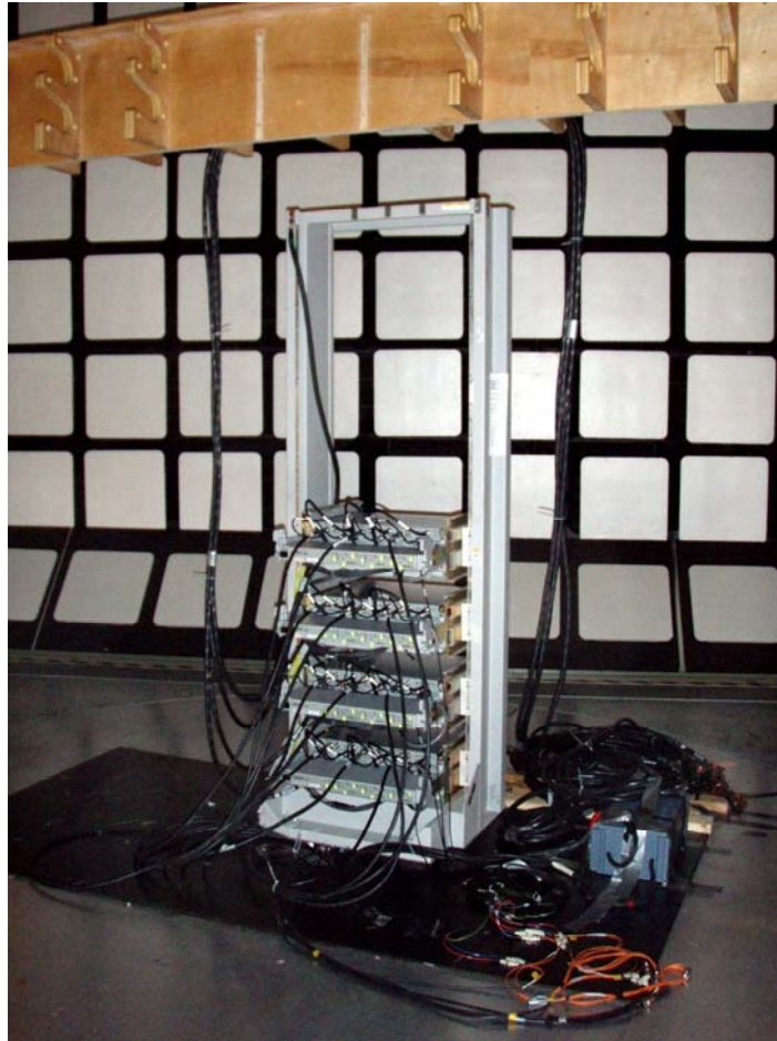
Figure 8-1: AWS 1.7/2.1 GHz MFRM-3 Beta Radiated Emission Set-up (Configuration 1 and 2 – Front View)
