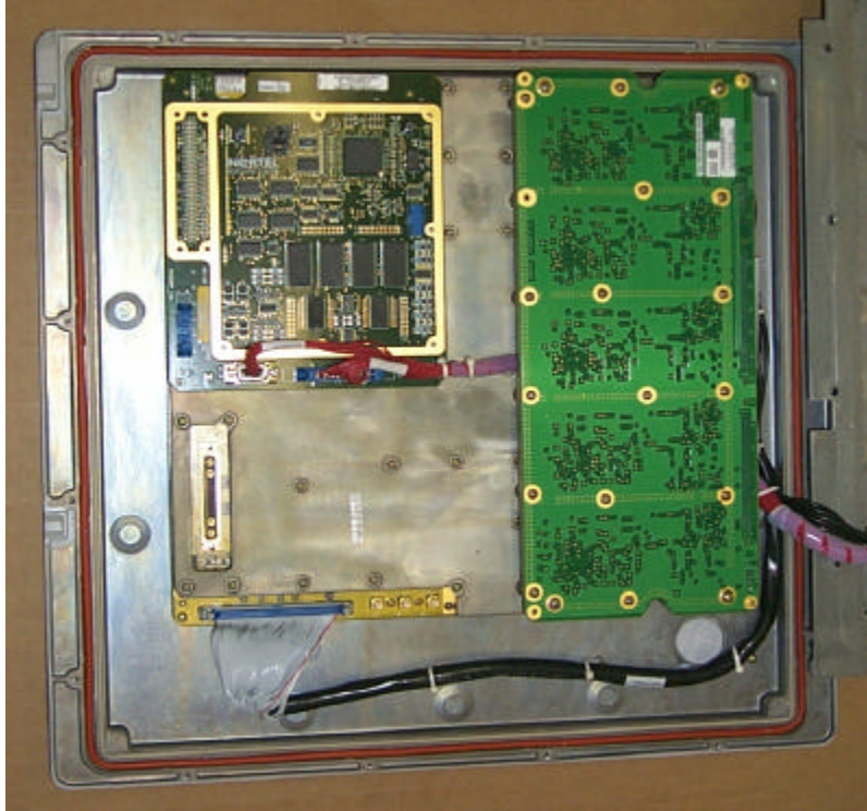
Figure 3: 1900 MHz TRM internal view
