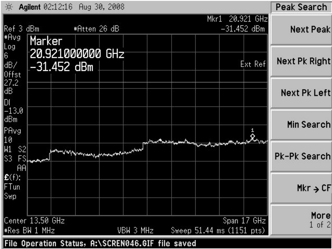
Figure 27: Spurious Emissions - 3 Carriers - Channel 1225, 1250, 1275, 5 GHz to 22 GHz
