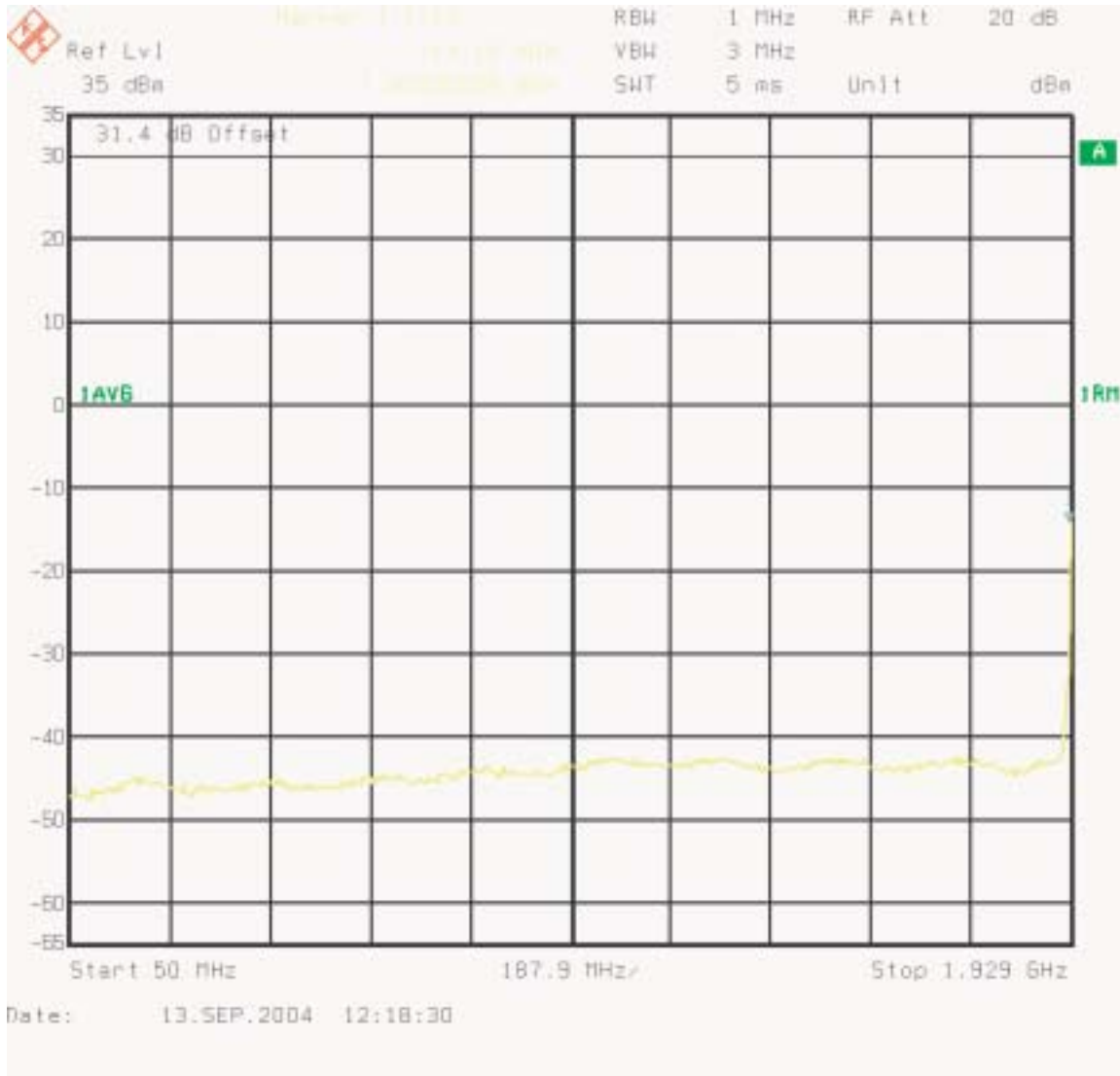
Figure 16 : Conducted Spurious Emissions - 3 Carrier, Chan 25, 50, 75 Two IS-95 One IS-856 QAM 16 (50 MHz - 1.929 GHz)
