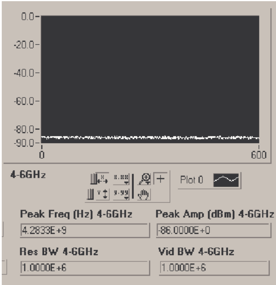
Figure 11 : Conducted Spurious Emissions - 1 Carrier, Channel 775 (4 GHz - 6 GHz)
