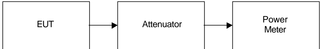
Figure 1 - Measurement Setup for RF Output Power
