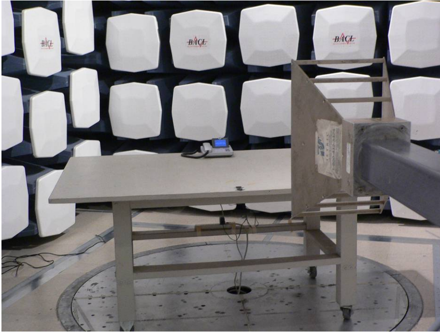
Radiated Emissions - Front View
