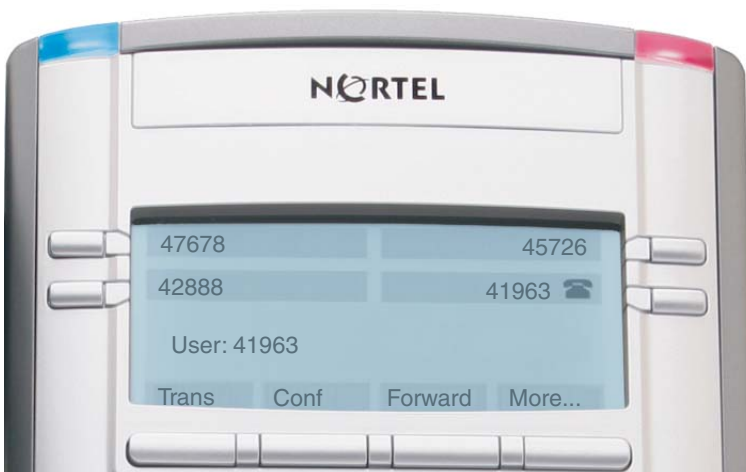
Figure 10: Logged in to an IP Phone 1150E using an IP Phone 1120E
