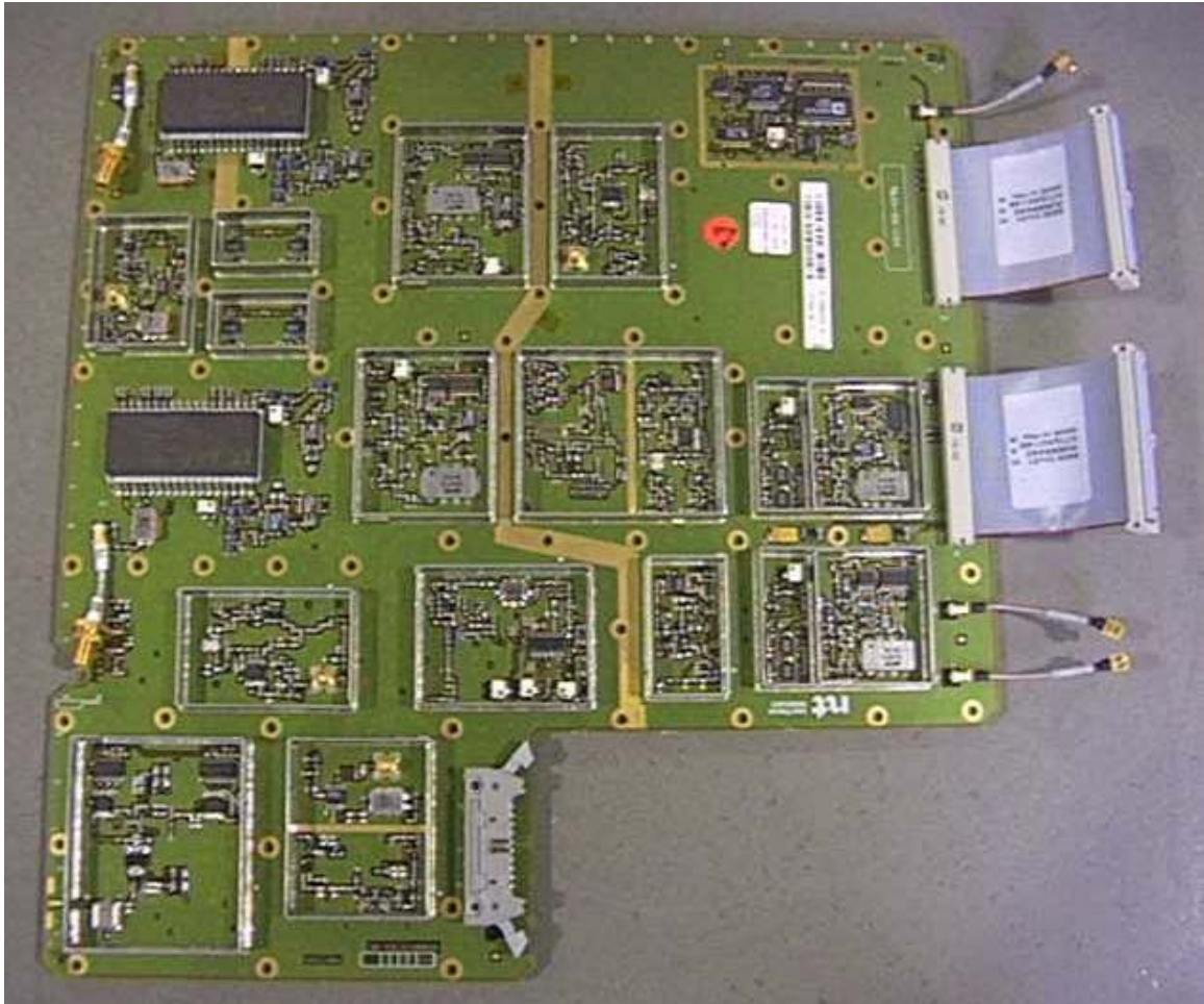
Figure 11 – RDRX 1900 MHz (Radio Board) Top View
