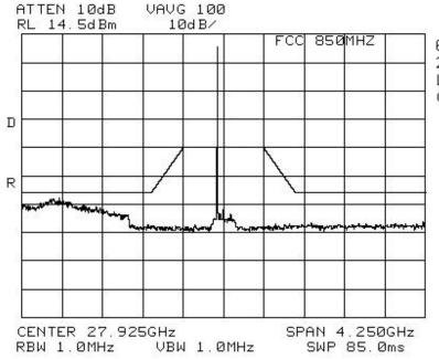
64 QAM, 1 Carrier 2.048Msps Lower Band Edge CTR 28-08M
