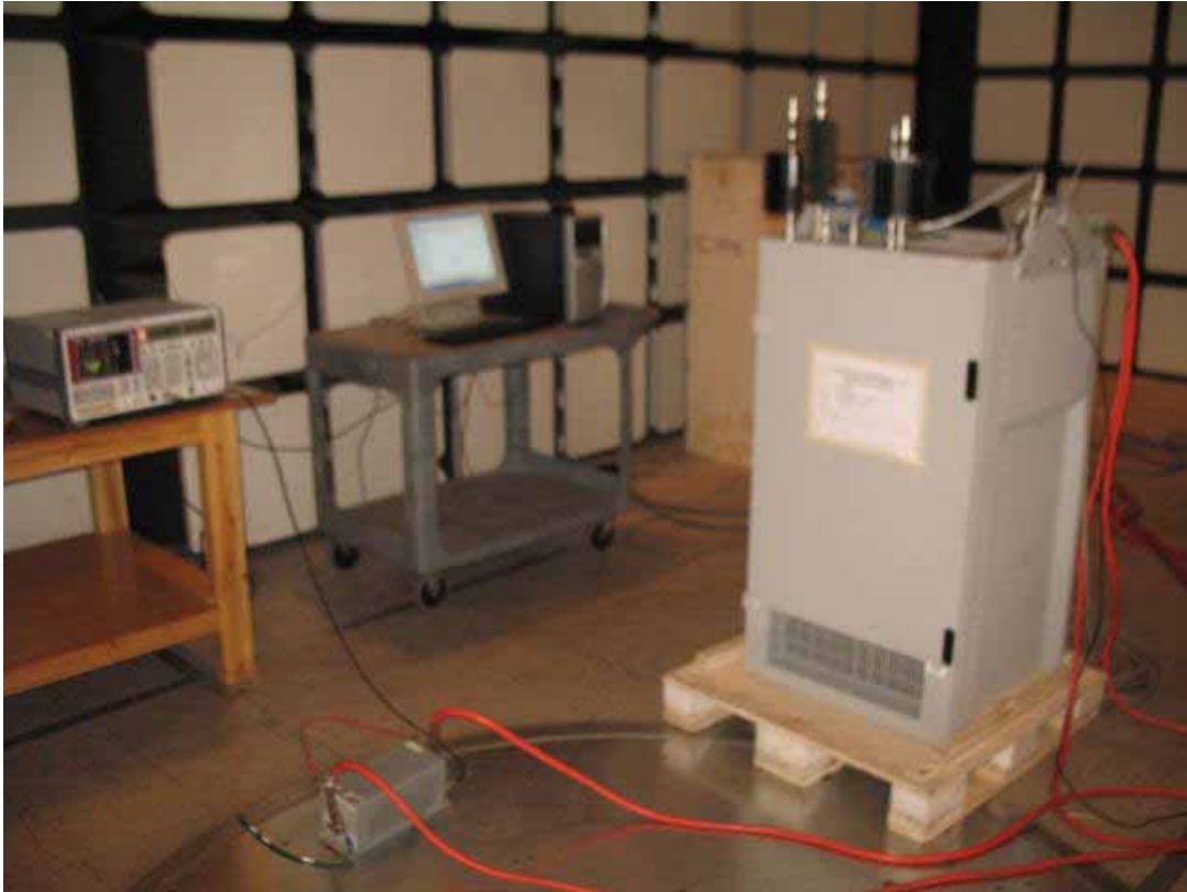
DC port Conducted Emission Test Set-up
