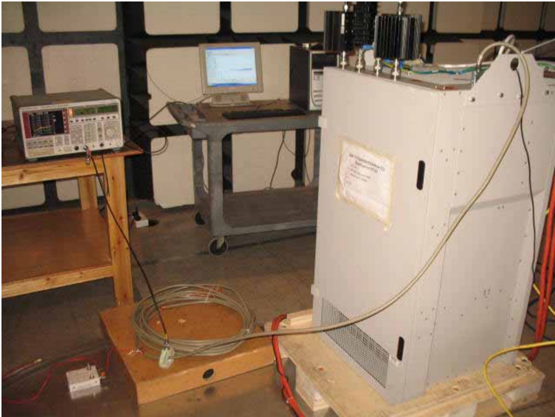
Conducted Emission at telecomm port Test Set-up
