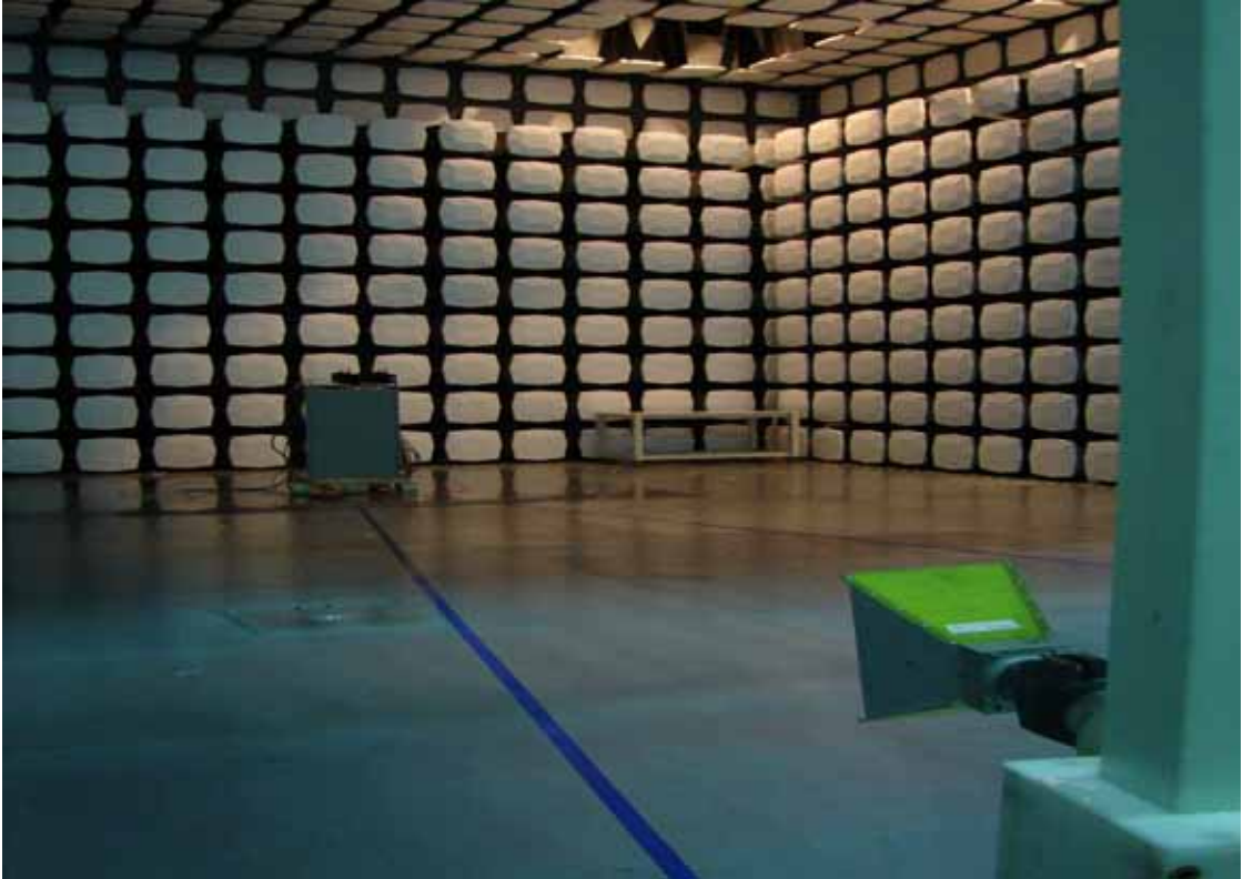
Radiated spurious Emission Test Set-Up 1G-18GHz
