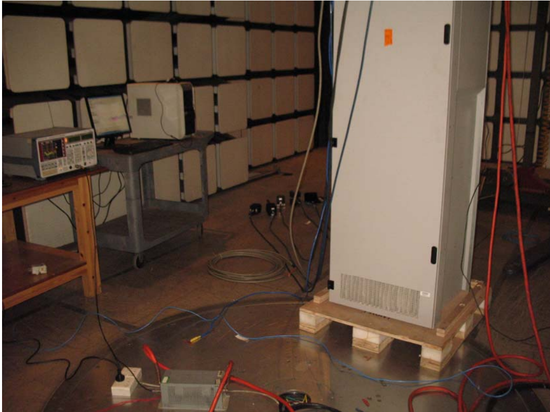
DC port Conducted Emission Test Set-up
